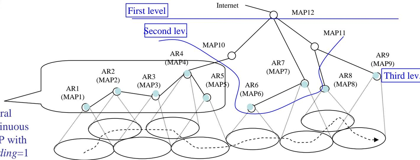
several continuous MAP with flooding=1 can be compressed as a hierarchy level.
