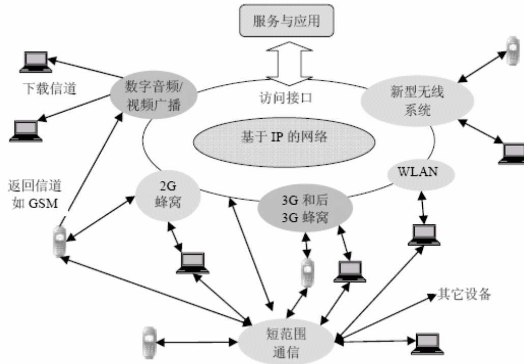
The integrated framework **based IP networks** of future heterogeneous wireless access networks
