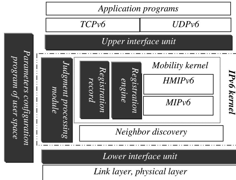
Fig. implementation skeleton diagram of AMMS
